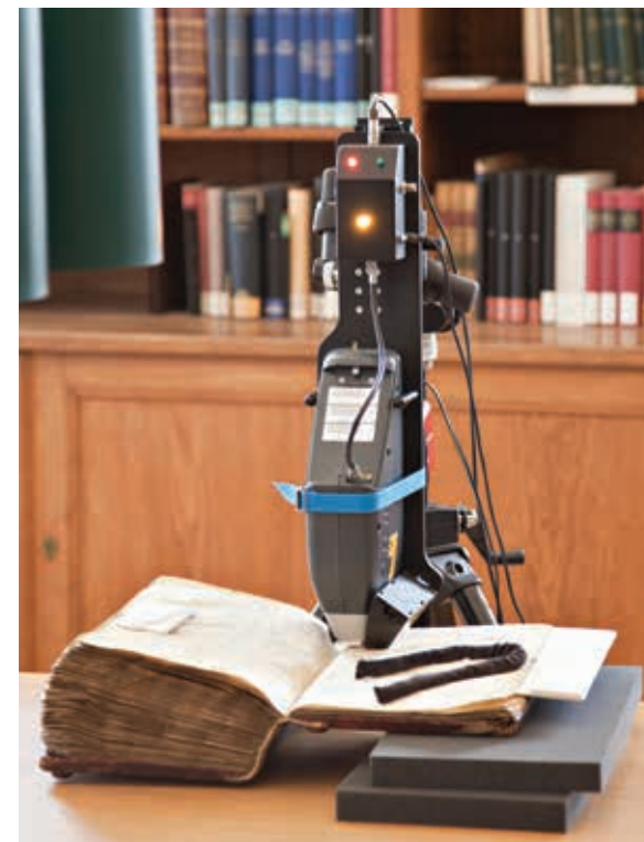
Fig. 2: The handheld instruments (Spectro XSort, Spectro Analytical Instruments GmbH., Kleve/Germany. www.spectro.com ) with a rather large spot size (ca. 3 mm in diameter)
