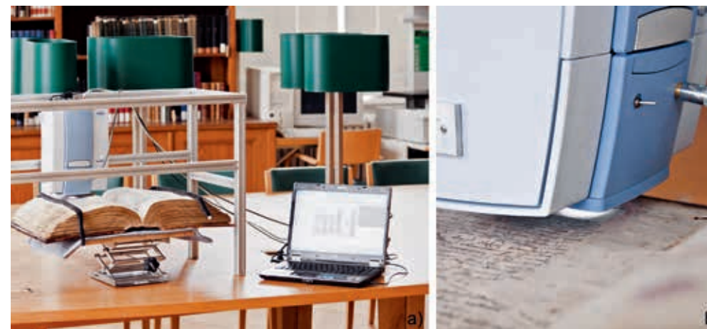
Fig. 3: rFTIR investigation with the Alpha spectrometer in the Austrian National Library, mounted on a four-legged stand (a). The distance between the rFTIR device and the object is about 15 mm during the measurement, thus contactless (b)
