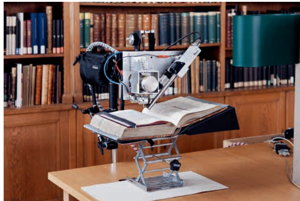
Fig. 1: XRF examinations with the pXRF, mounted on a tripod in the Austrian National Library. The measuring point is focused with the help of two laser pointers that are attached to the device. The distance between the XRF device and the object is around 15 mm during the measurement and is therefore contactless
