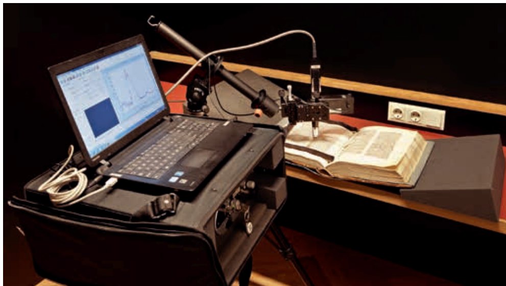
Fig. 4: Raman setup with the Enwave spectrometer in the Austrian National Library. The distance between the Raman device and the object is about 8 mm during the measurement guaranteeing a non-invasive and contactless analysis
